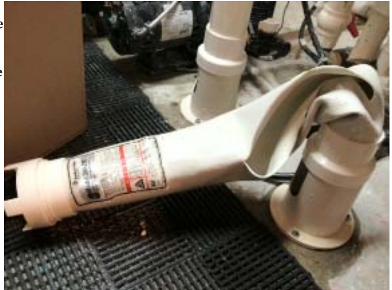
Erosion feeder designed for use with stabilized chlorine tablets melted and burst spilling the highly concentrated solution of liquid chlorine.
