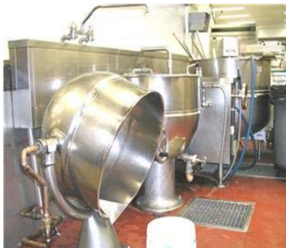
An acceptable non direct steam jacketed kettle. Usually an indicator a steam box may also be in use.
